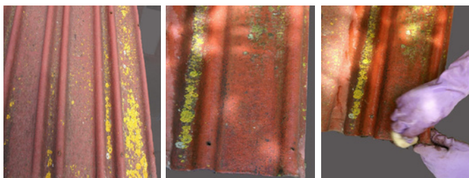
FIG 1 - Lichen on ONDULINE® sample
