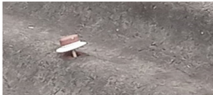
FIG 7 - Small oblong hole (less than 1cm 2 )
